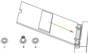
Align and gently insert the M.2 SSD module into the M.2 slot. Please be aware that the M.2 SSD module only fits in one orientation.
