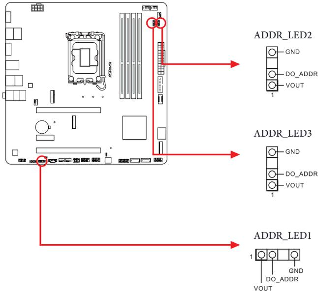
Connect your Addressable RGB LED strips to the **Addressable LED Headers (ADDR\_LED1 / ADDR\_LED2 / ADDR\_LED3)** on the motherboard.
